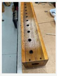
The pipe pneumatics of the Salicional Celeste offset chest with evidence of water damage and leather overlay technique.
